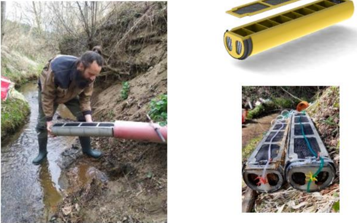
Fig. 1. Cartridge, location at drain pipe exit, and the experimental set-up.
