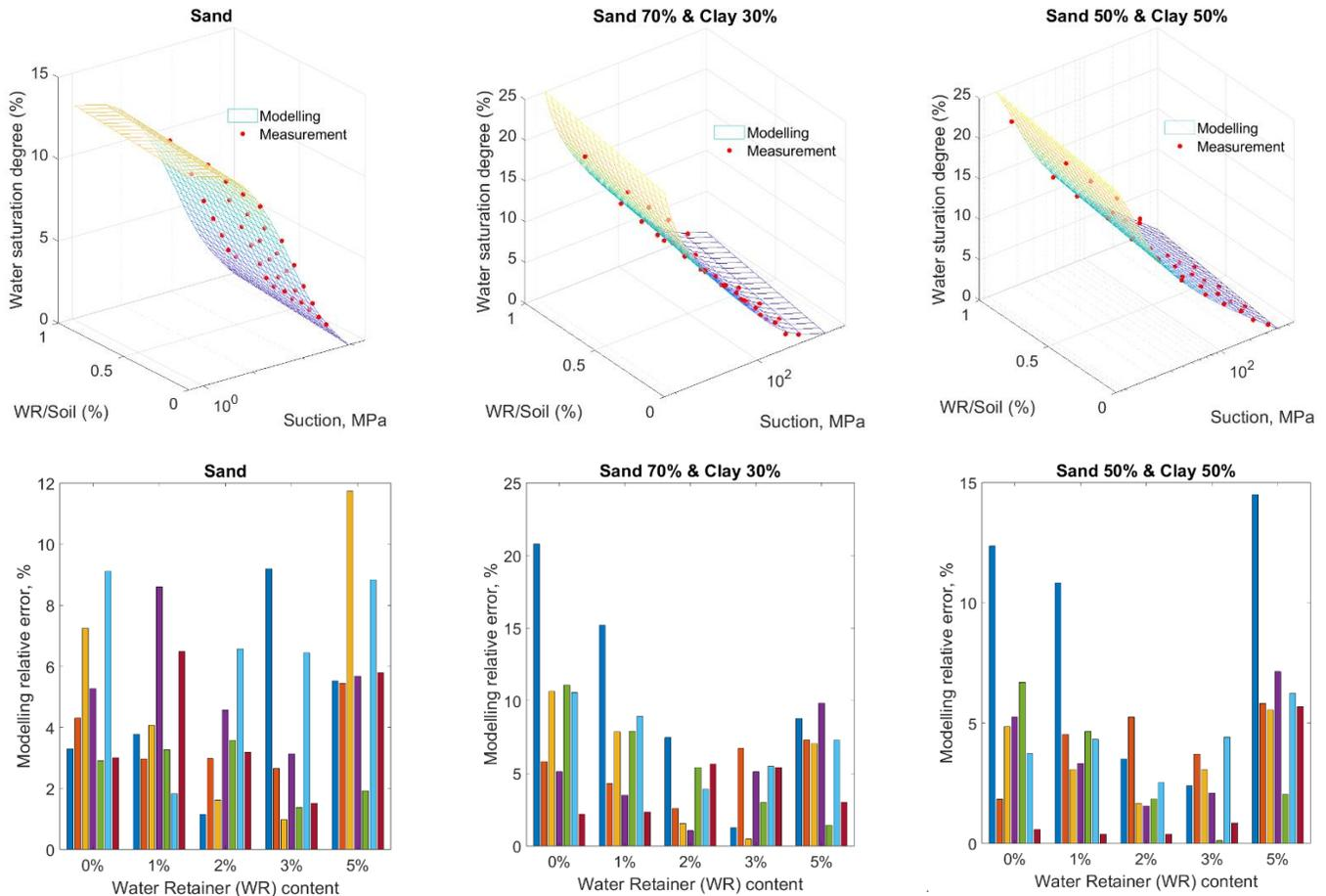
Fig. 6. 3D representative, the Eq. 1, for the water retention characteristic at different suction and water retainer percentage and the modelling error
