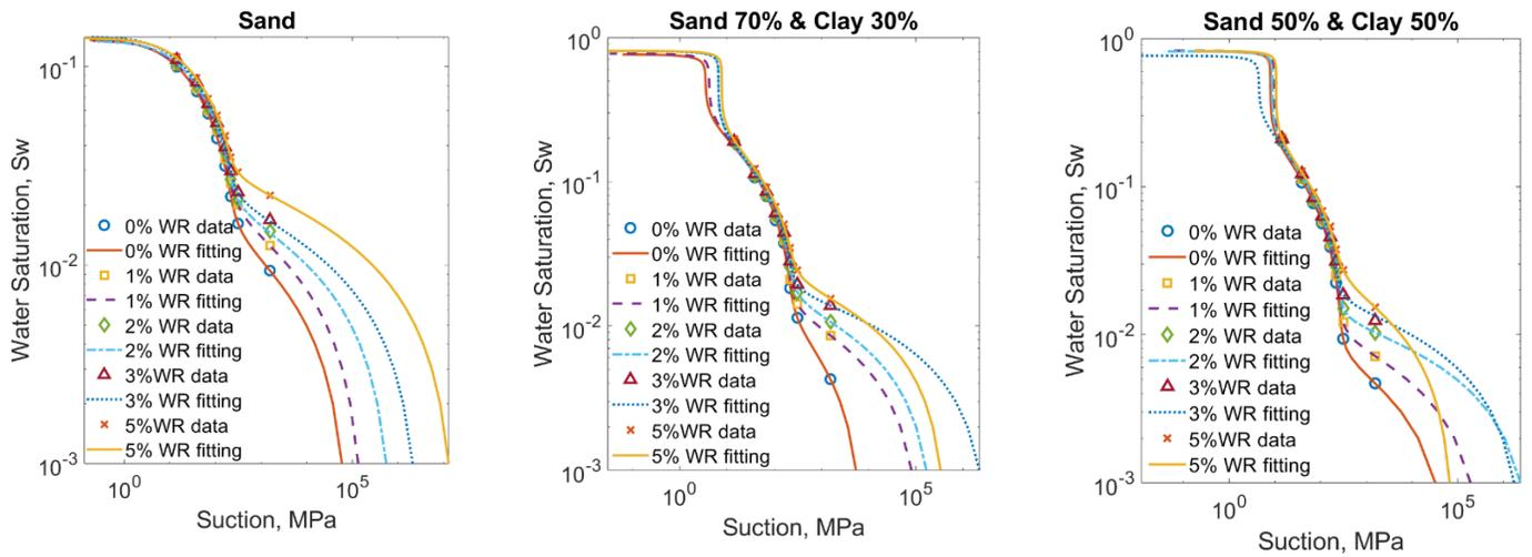
Fig. 2. Modelling results of Eq. (2) for the soil water retention curves
