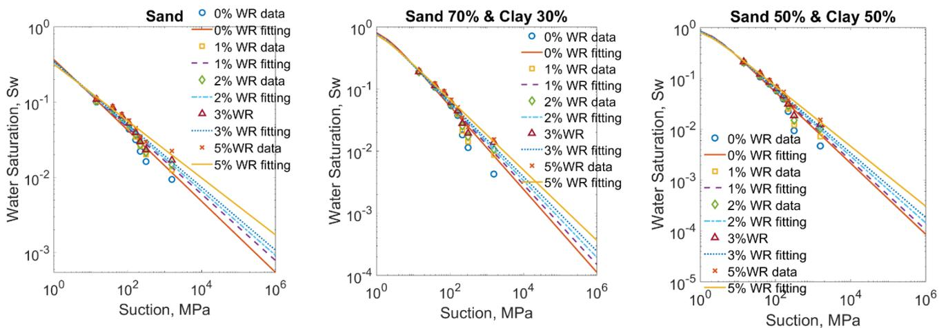
Fig. 3. Modelling results of van Genuchten model [2] for the soil water retention curves
