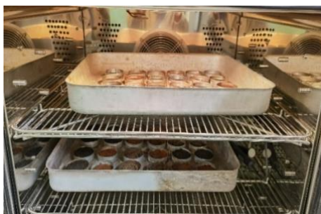
Figure 25: Experiments to determine soil hydraulic properties, (a) water retention test, (b) water diffusion test.
