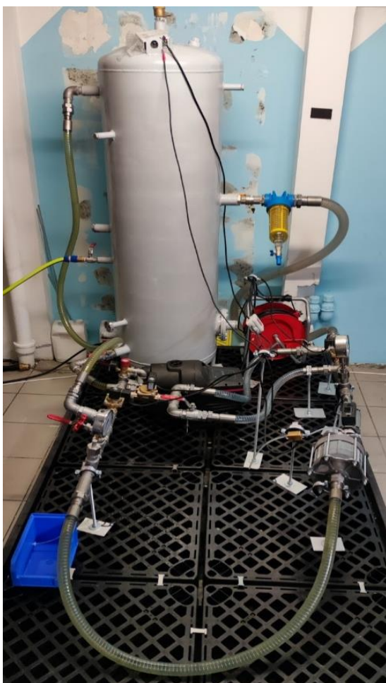
Figure 6. The lab scale experimental setup and the flow chart of the microfluidic nutrient recovery system; MV1, MV2, MV3, MV4A, MV4B, MV5: Manual valves; P1: safety relieve valve (3 bar); P2, P3: Manometer; NO1, NO2: normally open valves; NC1, NC3: normally closed valve; Q1: Flowmeter; Air: air bubble purge; CB: concentrated beads; SV: safety filter.
