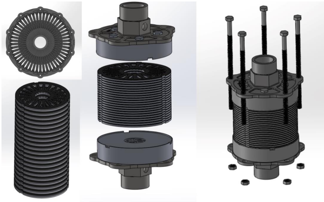
Figure 4. Microfluidic CD and its stackable design.
