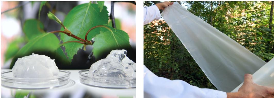
*Figure 1. The appearance of cellulose nanofibrils (CNF) or nanocellulose (left) and the produced cationic nanocellulose-based nutrient-collecting membrane (right).*
