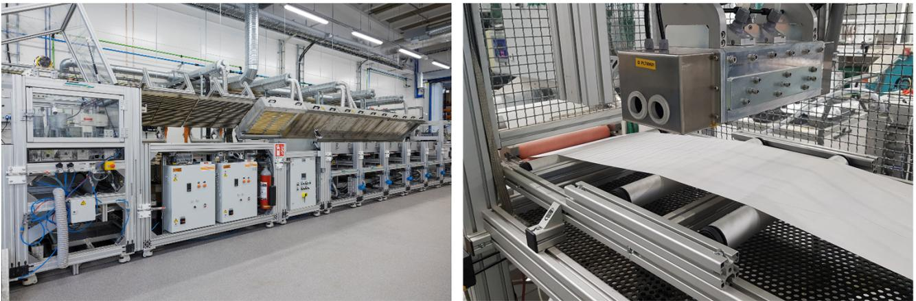
*Figure 2. Modular, R2R, pilot-scale commercial converting line (SutCo) for nanocellulose membrane preparation (left) and atmospheric plasma enhanced chemical vapour deposition unit for surface cationisation of already assembled nanocellulose membranes (right).*
