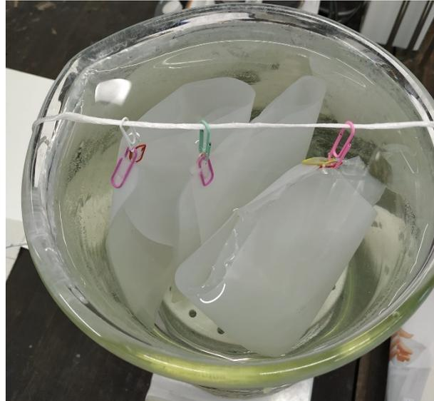
Figure 4. Nutrient uptake capacity measurements of prepared membranes
