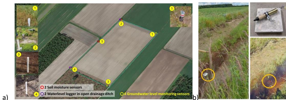
*Figure 6. a) The picture shows locations where groundwater level monitoring pipes, soil moisture sensors, and water level loggers in the drainage ditch were installed at the Tyrnävä field scale. b) water level loggers installed in the main drainage ditch of the case study area (WATERAGRI project).*
