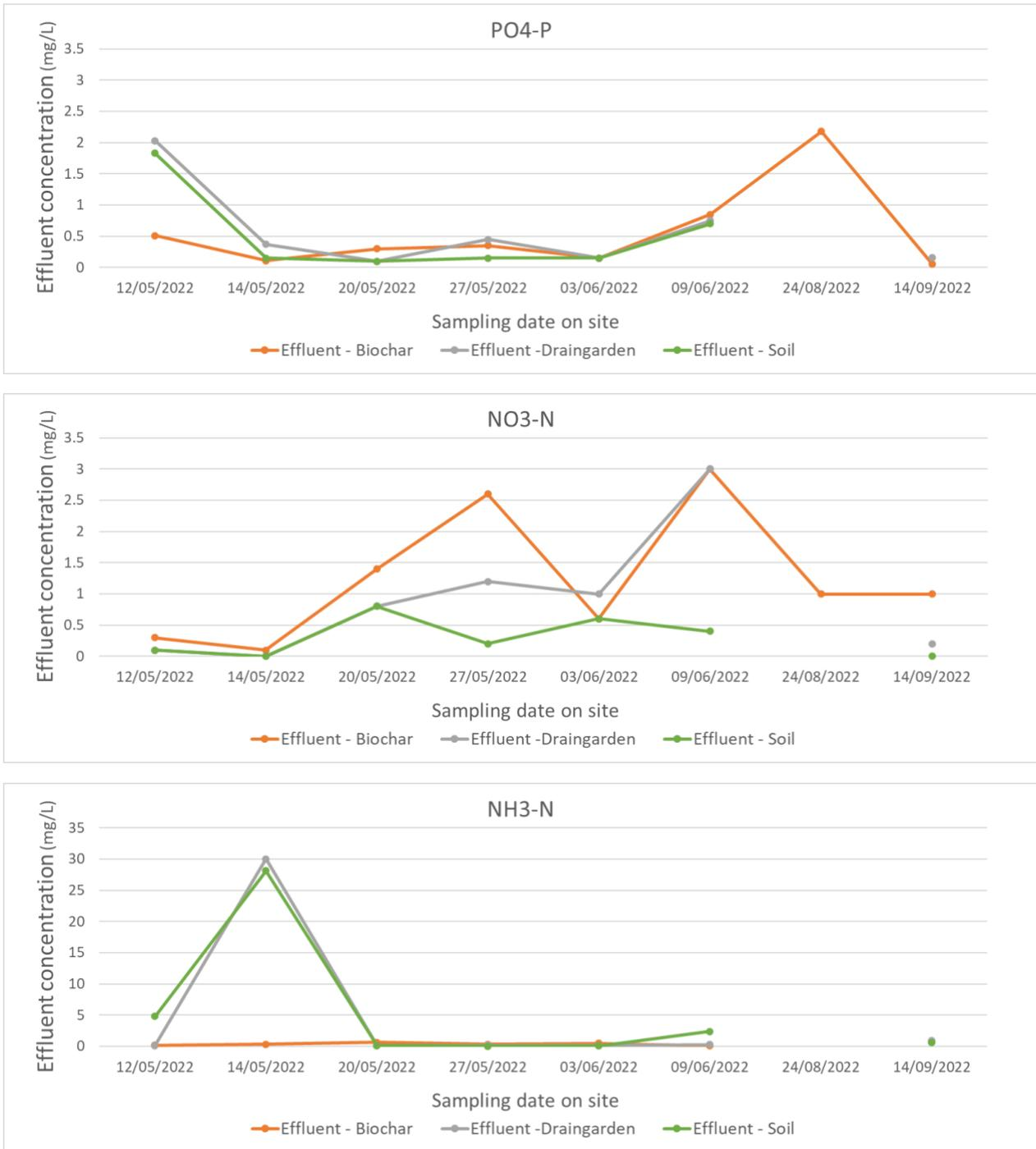
Figure 22. Effluent concentrations over time for PO<sub>4</sub>, NO<sub>3</sub>-N, NH<sub>3</sub>-N, Mistelbach pilot study case (The visit dates where no effluent was found are not shown).
