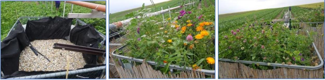
09.06.2022 Top view of the filters, from left to right: unvegetated biochar filter, vegetated soil, and vegetated Draingarden filter.
