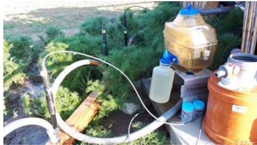
*Figure 17. Tracer experiment on 12.05.2022, three EC meter probes were placed in effluent cells and measured for 48 hours the effluents' electrical conductivity.*
