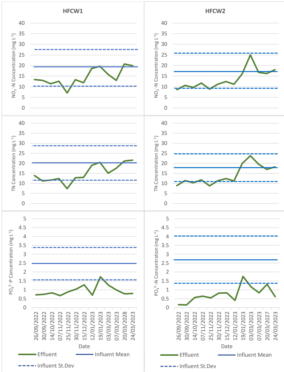
Figure 6 - Concentrations of nutrients in influent (mg L -1 , average ± standard deviation) and effluent of HFCW1 and HFCW2.
