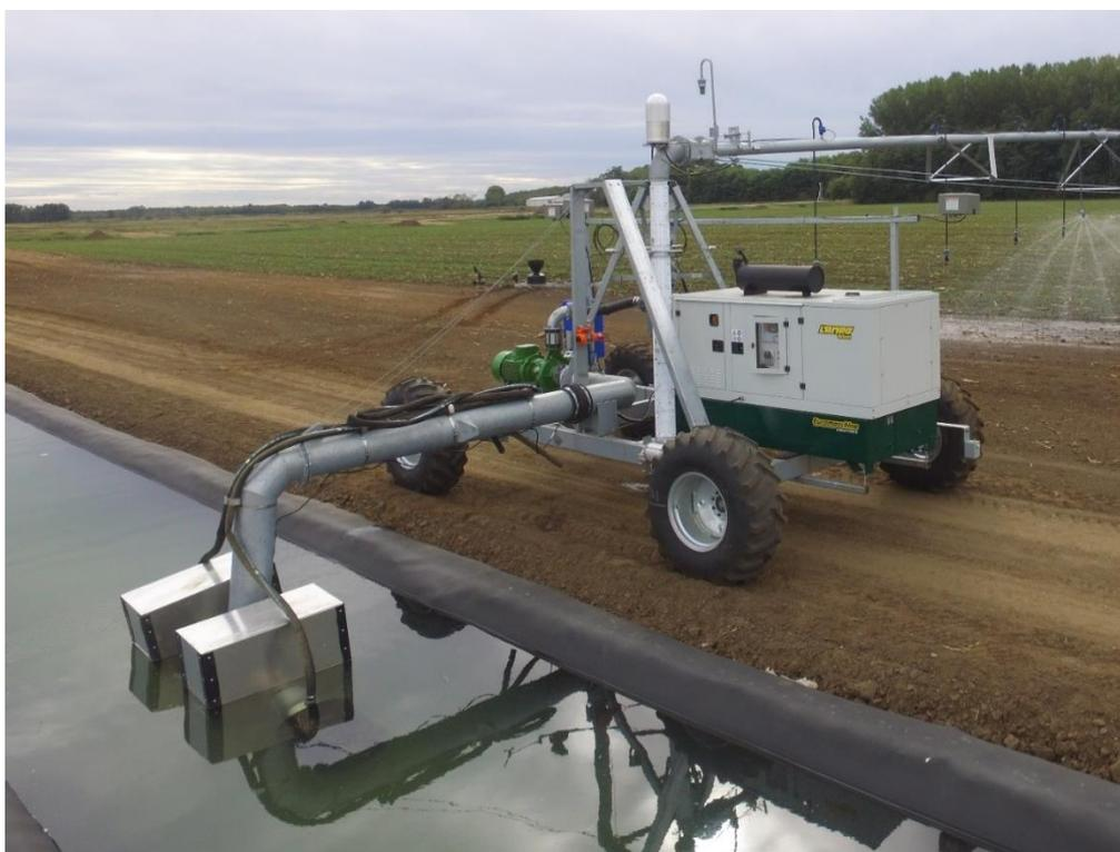
Figure 20. Four-wheel canal feed power cart
