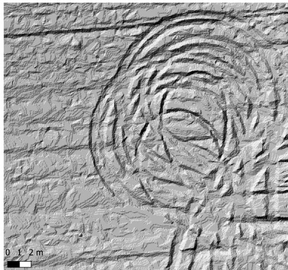
Figure 13: 2 cm DTM created from dense point cloud.
