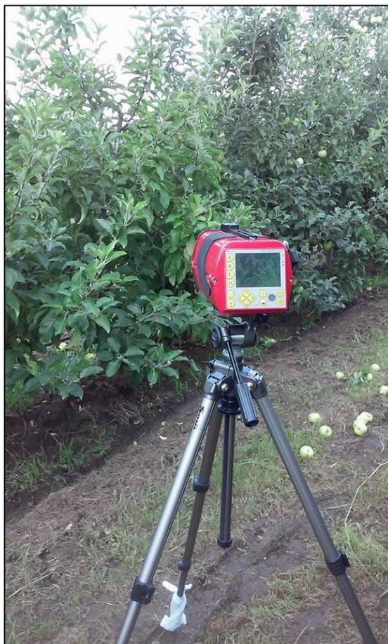
*Figure 10. Examination of the moisture content of apple foliage by means of a thermographic device (Hungarian example at the case study site)*
