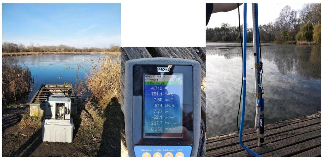
Figure 15. Water sampling from surface water body and in situ physico-chemical measurement
