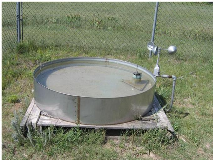
Figure 5. 'A' type evaporation pan (13)
