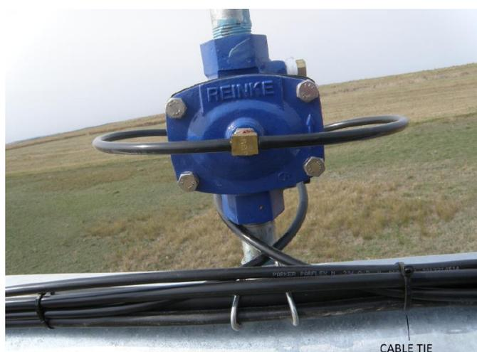
Figure 22.  $\frac{3}{4}$ " valve for sprinkler control
